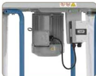
Powerful motor guarantees constant level of extraction at continuous operation.
