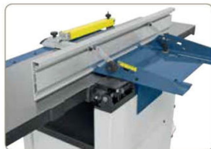
Solid planing fence with wide guide, tiltable from 90° to 45°.
