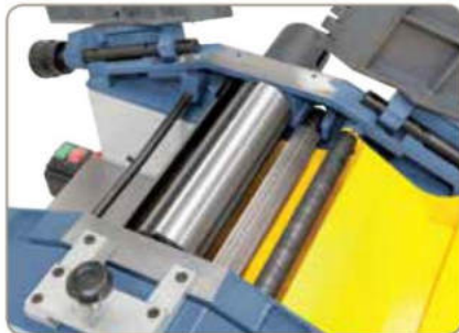
The planing unit consists of a 3-knife cutterblock, a corrugated infeed roller and rubber-coated outfeed roller.
