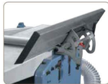
The planer fence can easily be adjusted from the back of the machine. The desired angle can be read on the scale.
