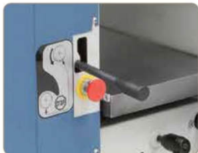
The infeed function can be switched off when planing.
