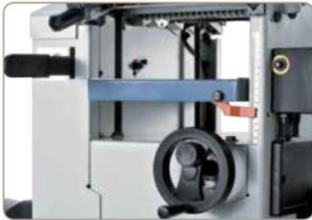
Thicknessing table is guided on four threads. The height can be read on the scale.
