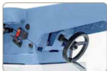
Quick and easy adjustment of chip removal (up to 8 mm).
