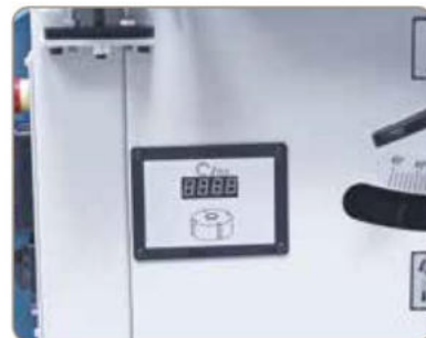
Electronic display of spindle speed settings.
