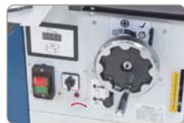
Electronic display of spindle speed settings.
