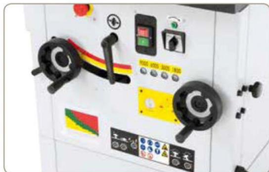
User-friendly position of controls elements, electronic speed display on LED indicator.
