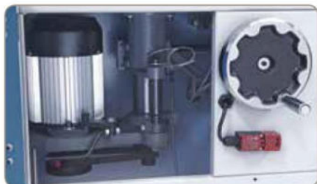
The large opening on the front of machine ensures quick and easy speed change.
