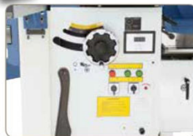
Electronic display of spindle speed settings.
