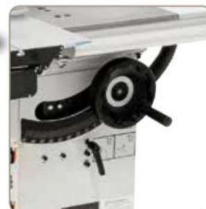
Sawblade angle can easily be read out on scale.
