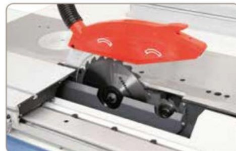
Sawblade cover with integrated dust port positioned at riving knife. Scoring unit is part of equipment.
