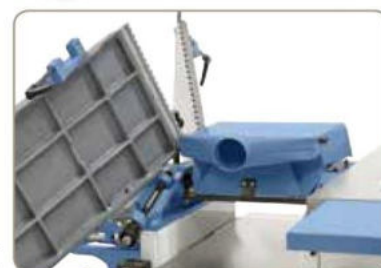
Integrated, tiltable dust hood - extraction outlet 100 mm.
