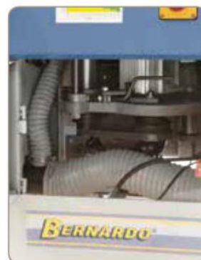
Oversize opening on machine front allows for easy belt change to adjust speed.
