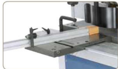
Grey, cast-iron roller table constructed and polished with top accuracy.
