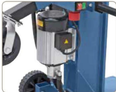
Powerful electro motor and high quality hydraulic pump.
