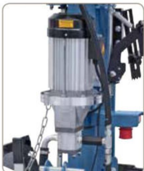
ZE-models with powerful electro motor and high quality hydraulic pump.
