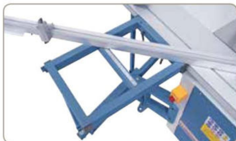
Generously sized square table for support of large sheet material.
