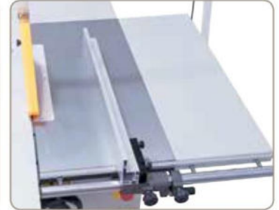
Parallel fence with quick and fine adjustment for cutting width up to 620 mm.
