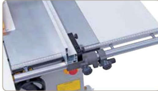
Complete with robust parallel fence, 30 mm round rod guide designed for heavy work loads.
