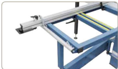
Square table with roll ensures convenient machining of large workpieces.
