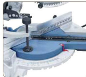
Rotary disc swivels 45° to both sides and features rests at 0° / 15° / 22.5° / 31.6° and 45°.
