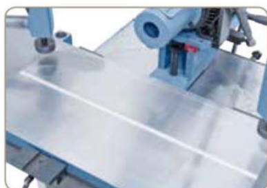
Drill table features scale with zero marking in the middle.
