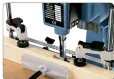
Eccentric clamp and quick clamping vice for secure fastening of workpiece.
