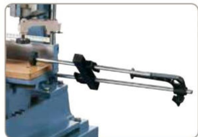
Convenient longitudinal fence for repeated operations.
