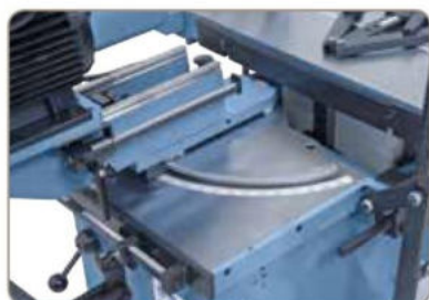
Drill head tilts 60° to right and left.
