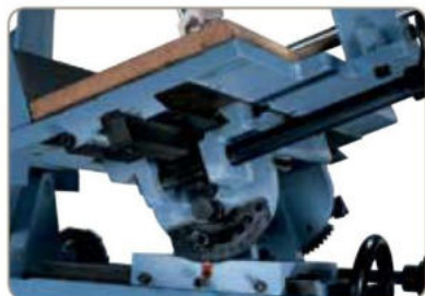
Work table tilts to front and back, which increases the range of applications significantly.
