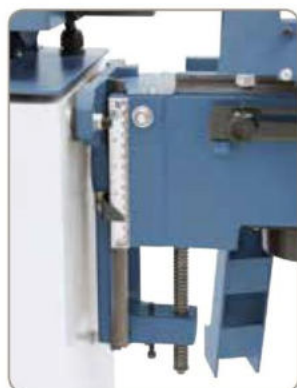
Set height of work table can be read out on scale.
