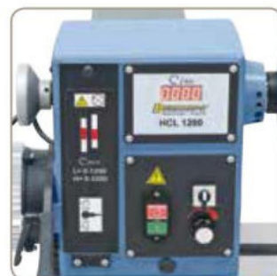
Digital display - as part of standard equipment - ensures comfortable, smooth speed setting.
