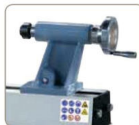
The compact tailstock can easily be locked into position by one-hand lever.
