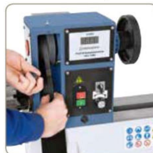
Repositioning the V-belt allows for easy change of the transmission ratio.
