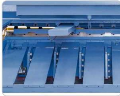
The pneumatic sheet support system (standard) prevents the bending of thin sheets and therefore ensures an exact cut.
