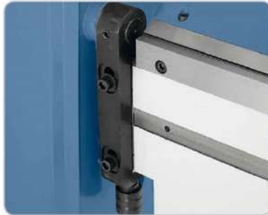
Manual adjustment of the desired sheet thickness by means of knurled screws.
