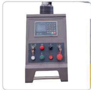
Integrated control NC-89 at the tiltable control panel.
