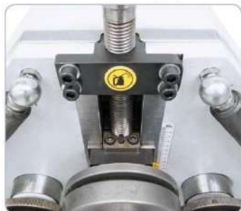
Stable guiding of the upper roll, adjustable via mm scale.
