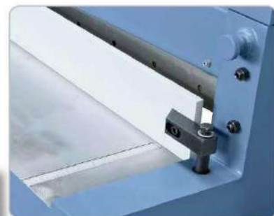
Inlaid measuring tapes in the work table.
