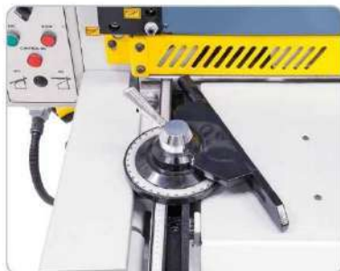
Optionally available angle shearing device for mitre cuts.
