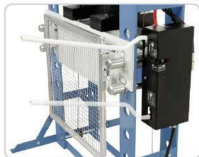
The piston stroke is carried out either by a hand lever (2 stages) or pneumatically by foot pedal.
