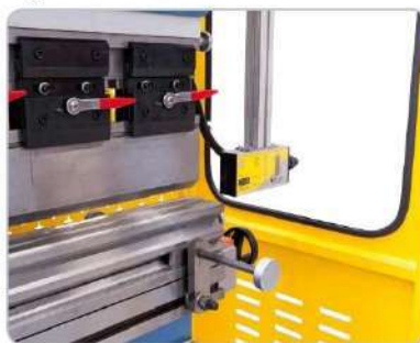
Non-contact, moving, laser-optical safety system Fissler AKAS-LC II.
