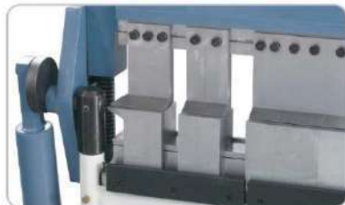
Segmented upper, bottom and bending beam for a large number of bending options.
