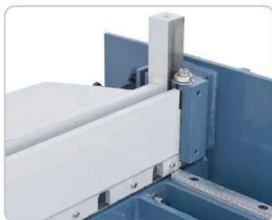
The robust rectangular guide guarantees optimal guidance of the upper knife.
