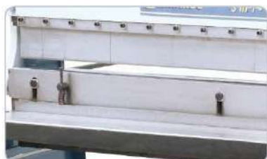
The removable inserts result in a high number of bending possibilities.
