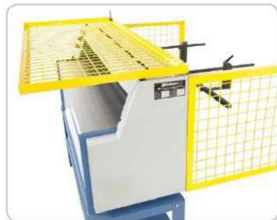
Hinged protective cover for easy removal of the finished workpiece.
