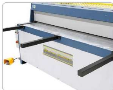
The support arms facilitate the processing of large format sheets.
