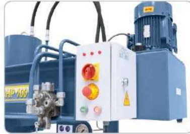
The control panel contains all important switching elements.
