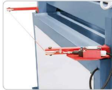
Increased safety through safety rope.
