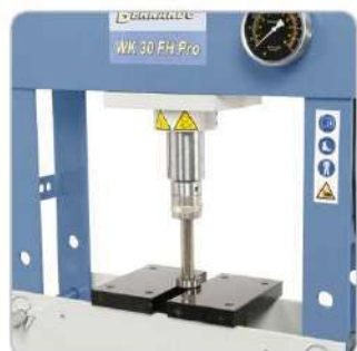
The optionally available pressure pin set additionally increases the field of application.
