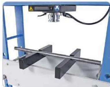
For straightening shafts, optional prism supports are available.
