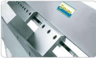
Due to the individually removable segments also boxes, cases, etc. can be bent.
