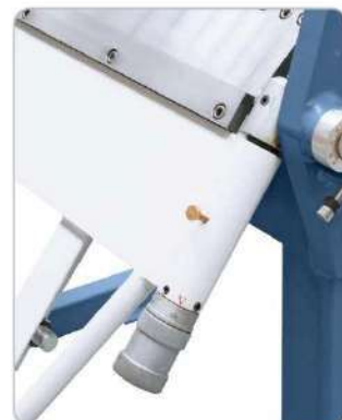
The setting of the desired material thickness is done quickly and easily by means of adjusting screw.
