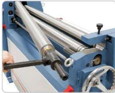
Adjustment of the bottom roller by handwheel, upper roller can be swivelled forward.
