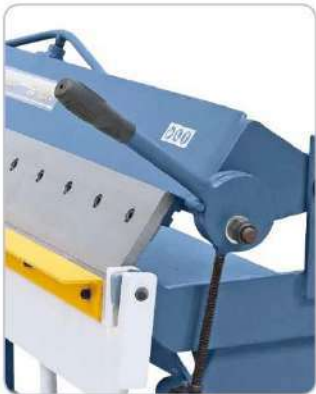
Easy lifting of the upper beam by lever.
