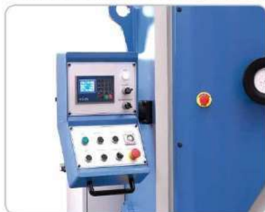
Integrated control NC 10 in the control panel, standard with memory function
