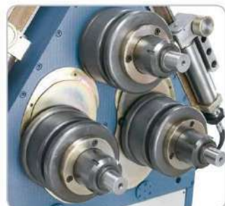
Hardened and ground rolls and shafts.
