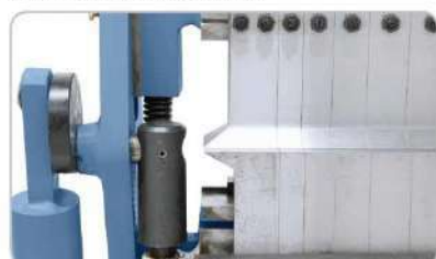
The lifting of the upper beam take place via an eccentric.
