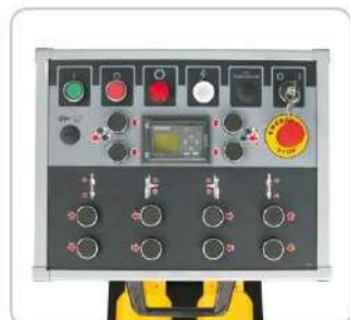
Control panel BPK 80 H with hydraulically adjustable guiding rolls (option).
