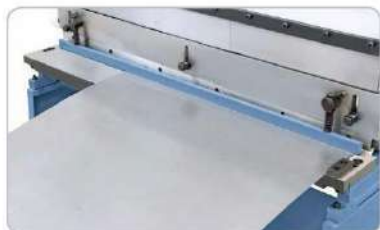
When cutting, the workpiece is automatically clamped.
