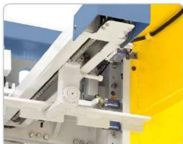
Backgauge with ball screw for increased accuracy.
