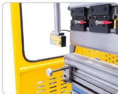
Non-contact, moving, laser-optical safety system Fissler AKAS-LC II.
