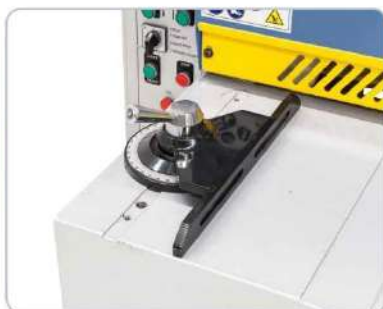
The optional angle shearing device allows miter cutting.
