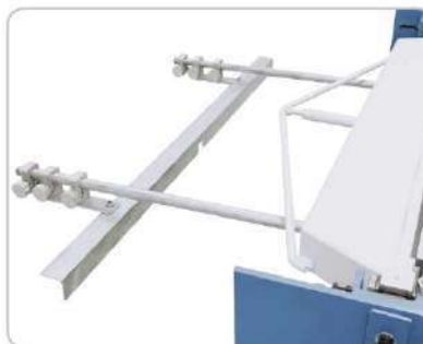
Robust backgauge, adjustable from 0 - 600 mm.
