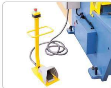
Operation by foot pedal, therefore both hands free for the workpiece.
