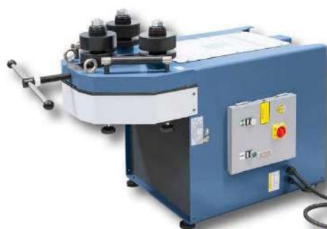
Stable guiding of the upper roll, adjustable via mm scale.
