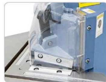
Protective cover out of Plexiglas, therefore optimal view to the cutting edge
