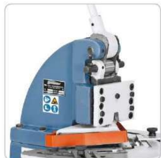
Mechanical power transmission by means of eccentric.
