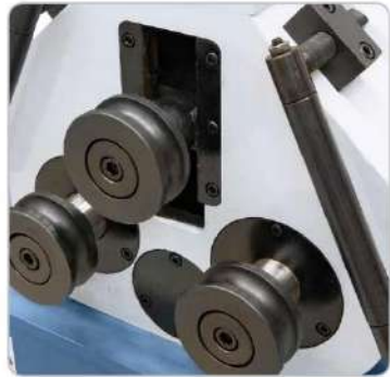
Guiding of the upper roll by precision ground guide rails.
