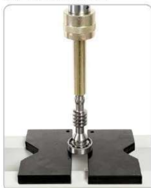
Extended range of application through the optional pressure pin set.
