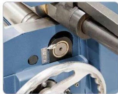
Exact adjustment of the bottom roll by scale.
