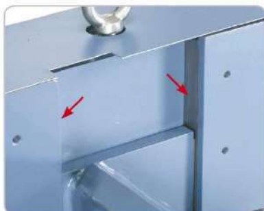
Large dimensioned guide guarantees exact bending.
