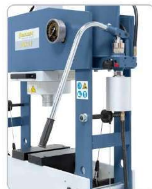
Large dimensioned lever for easy infeed of the pressure piston.
