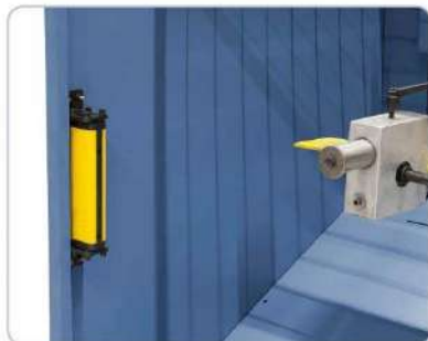
The standard light barrier prevents intervention in the running machine.
