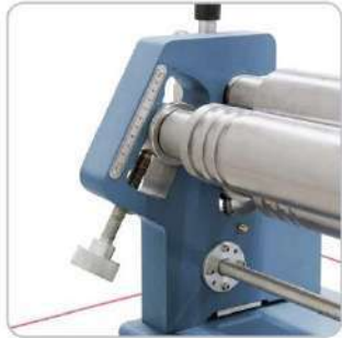
Exact adjustment of the back roller by scale.
