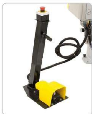
Separat foot pedal with integrated emergency stop button.
