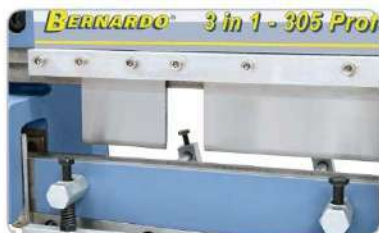
Due to the individually removable segments also boxes can be bent.
