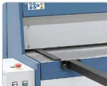
Exact, right-angled adjustment by lateral stop.
